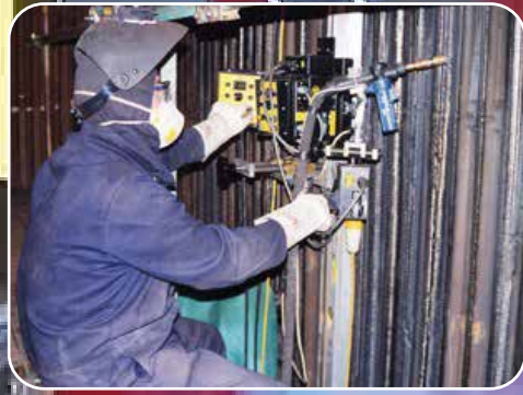
Position Overlay System
